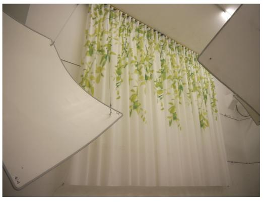
Figure B.2. Folded arrangement, test object mounted in the reverberation room.
