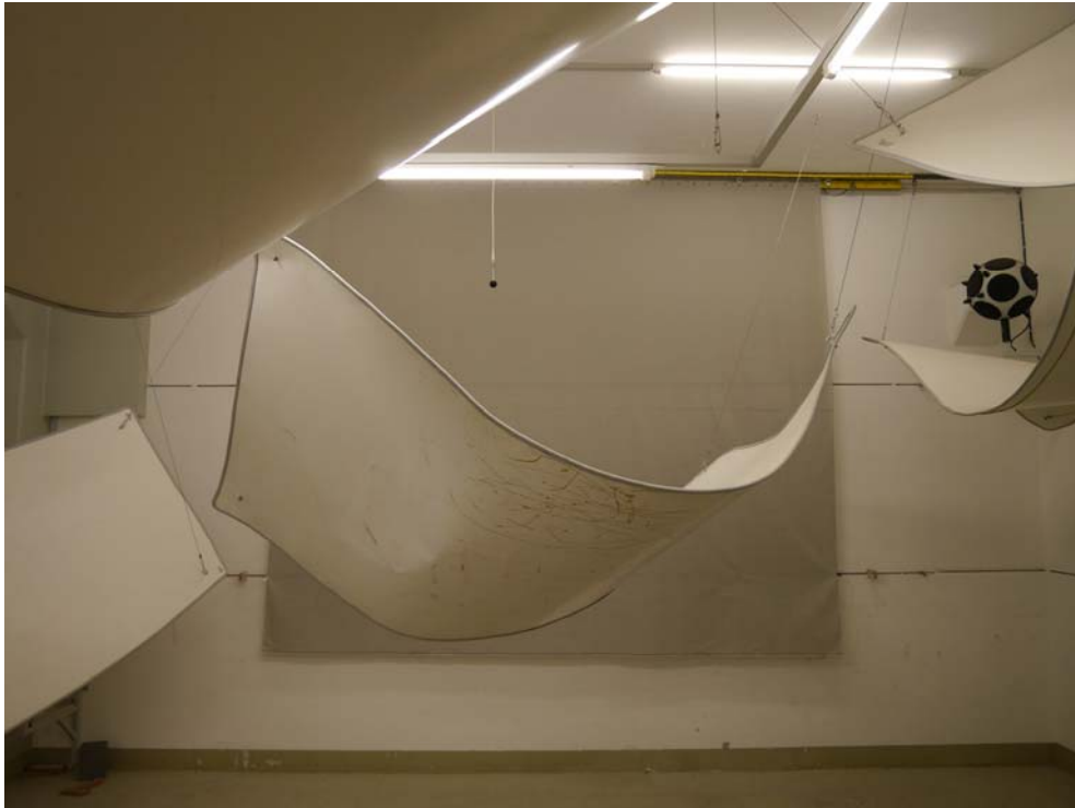
Figure B.1. Test object mounted in the reverberation room (frontal view).
