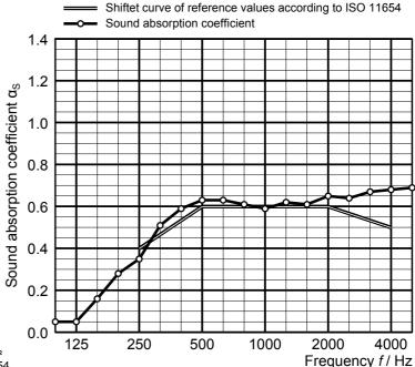
$<sup>\</sup>circ$  Equivalent sound absorption area less than 1.0  $m^2$   $\alpha_S$  Sound absorption coefficient according to ISO 354
