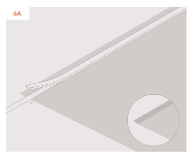
For Fabrics less than 3mm thick: Apply the Insert Bead up to 1/2" below the top edge of the fabric. Working in short sections, remove the liner and apply the Insert Bead up to 1/2" below the top edge of the fabric, pressing down firmly to secure it. Fold the top edge of fabric over the Insert Bead once. Note: If fabric has a lot of negative space/openings make sure to apply the Insert Bead to an area with the least amount of negative space.
