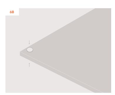
For Fabrics 3mm-6mm thick: Insert the Rivets into holes at the top of the fabric panel; two pieces are used for each hole.
