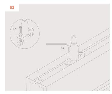
Attach the Bar Mounts to Bar: (3A) Loosely attach the T-nuts to the bottom of the Bar Mount using the #3 Bolts. (3B) Slide the Bar Mounts into the Bar to desired location and tighten the Bolts using the 2mm Allen Wrench.
