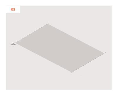
Cut fabric to desired length; ensure cut edge is square to the fabric and does not have excessive fraying.
