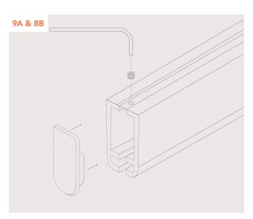
Install the End Caps at both ends of the Bar fixture and tighten Set Screws using the Allen Wrench.
