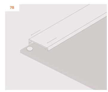
Insert/Slide top of fabric panel, with the Rivets, inside the Bar fixture so the fabric panel is hanging through the gap.
