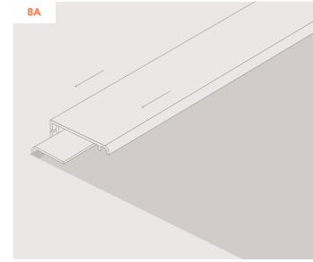
Insert the assembled Gripper Strip with fabric into one end of the Bar fixture so the fabric is hanging through the gap.
