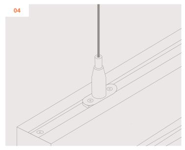
Determine the desired length of the cables and cut to approximate length plus 1". Insert one end of the cable into the Ceiling Mount. Insert the other end to the cable gripper on the rail mount. Adjustments can be made by compressing the locking mechanism on either mount. If there is excess cable, it can be left inside the Bar Mount and channel at the top of the Bar. Repeat steps 3 and 4 if a bottom Bar is being used. If the bottom Bar needs to be fixed to the floor, follow steps 1 and 2.
