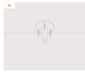
Use (3) #6 screws to attach each Ceiling Mount to the ceiling.
