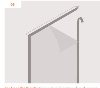
For Liner (Optional): Remove tape from the velcro along one edge of the liner. Starting with a corner, apply the edge of the liner, adhesive down, to the inside channel. Repeat until all 4 sides of the liner is applied to all 4 sides of the channel.
