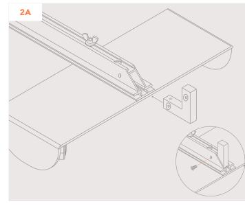
Insert and secure an L Bracket on each end of the Short Extrusion. Insert a Hex Screw into the hole on the side of the Short Extrusion and loosely secure the L Bracket.
