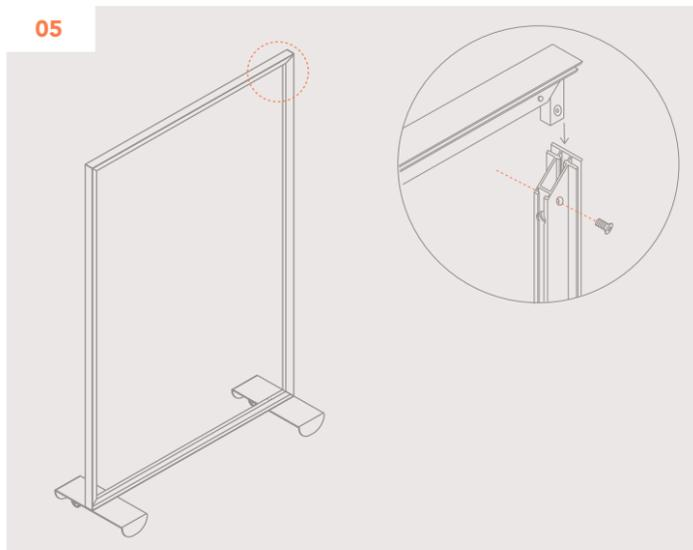
05 Insert the assembly into the Long Extrusions and secure the Hex Screws using the Allen Key.
