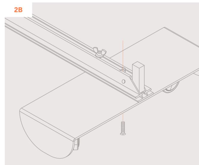
Insert a Short Screw through the bottom of the Base into the L Bracket.
