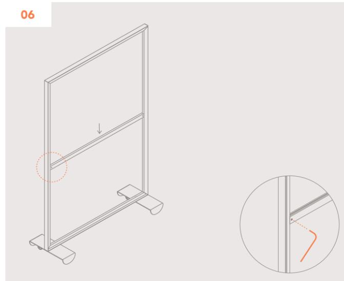
06 Insert the Support Bar into the Long Extrusion channels and tighten the screws using the Allen Key to keep the bar in place. *If no acoustical substrate or liner is being used, proceed to step 9.*
