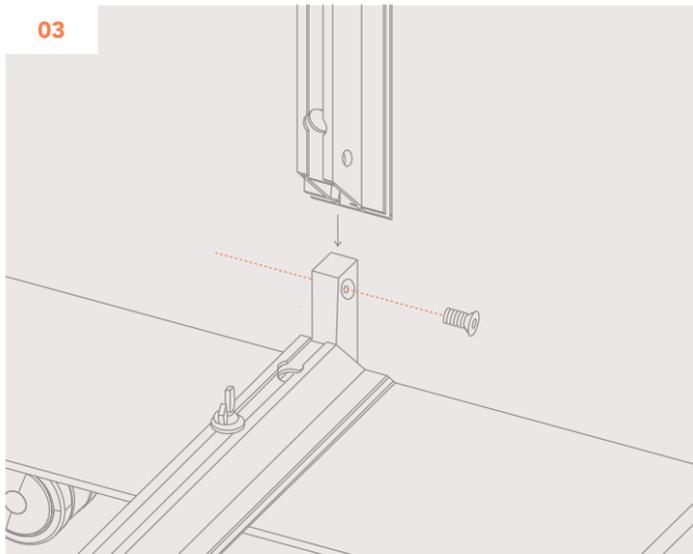
03 Insert the Long Extrusion onto the exposed end of the L Bracket and secure using the Hex Screw and Allen Key. Repeat this step on the other side.
