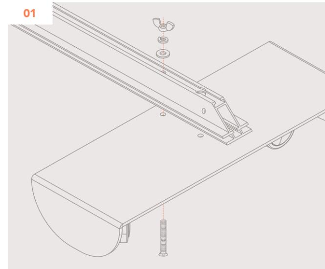
Attach a base to each end of one Short Extrusion using the long screws, plain washer, split nut washer and wingnut.
