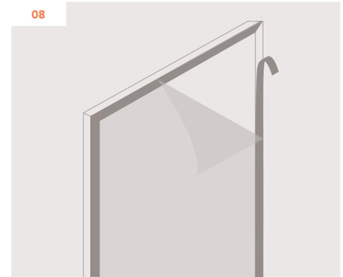
08 **For Liner (Optional):** Remove tape from the velcro along one edge of the liner. Starting with a corner, apply the edge of the liner, adhesive down, to the inside channel. Repeat until all 4 sides of the liner is applied to all 4 sides of the channel.
