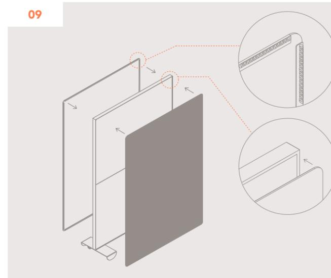
09 Install textile skins by guiding the silicone bead into the frames channel. Secure corners first and work around the frame.
