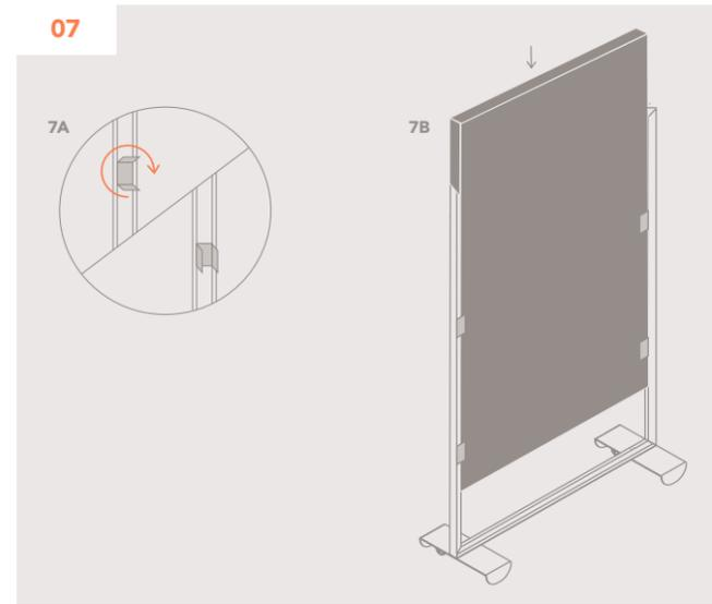
07 **For Acoustical Substrate (Optional):** 7A: Insert a clip into each Long Extrusion channel on the lower part of the frame. Turn clip gently to lock it in place. 7B: Carefully and slowly slide the substrate into the clips, pushing the substrate into the screw and wingnuts at the bottom of the frame. Repeat 7A and 7B for the 2 remaining substrate sheets. Adjust the Support Bar as needed.
