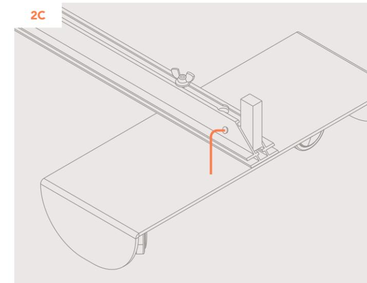
Use the Allen Key to tighten the Hex Screw that was inserted for Step 2A.
