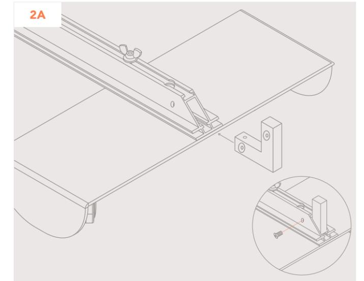
Insert and secure an L Bracket on each end of the Short Extrusion. Insert a Hex Screw into the hole on the side of the Short Extrusion and loosely secure the L Bracket.
