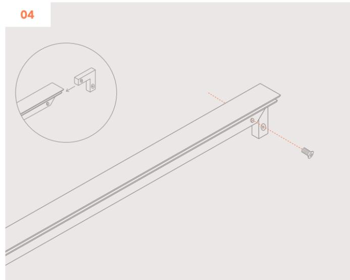
04 Attach the remaining set of L Brackets by sliding them inside the ends of the remaining Short Extrusion and loosely secure them with Allen Key and Hex Screws.
