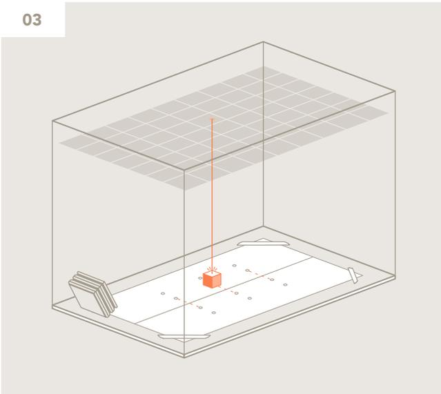
Using either the stickers provided or tape, begin marking the anchor points on the floor using the (E) measurements, directly under the location the baffle will be installed. Repeat until each baffle is accounted for.
