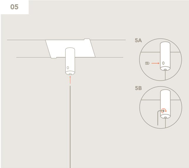
Insert one end of the cable into the pendant attached to the T-Bar clip. Secure the cable using the setting screw and allen key.
