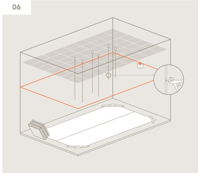
Set the wide field laser at the C measurement and cut each cable. Reference chart within this guide for the (B) measurement of the shape and size baffle being installed. Calculate the sum of the (B) measurement and desired finished suspended baffle baseline height (A). Once determined (B+A) subtract that number from current ceiling height, this will determine the cut length (C) of the installed cables.
