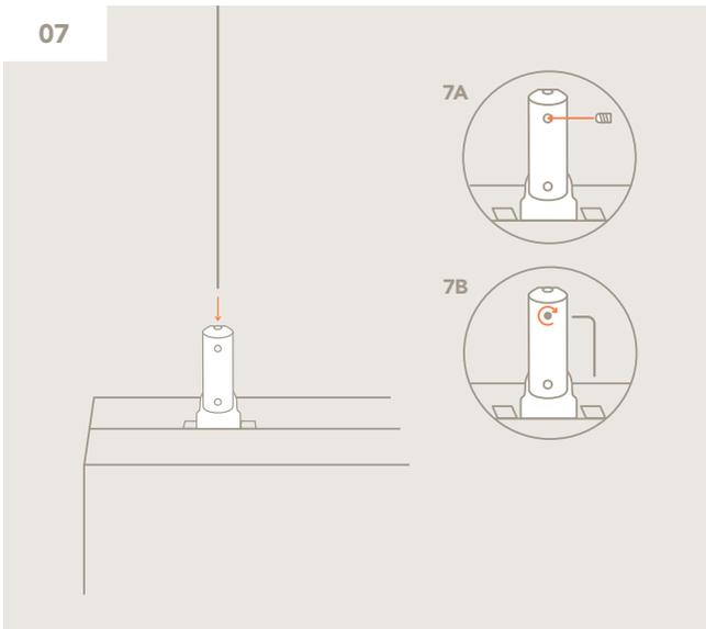
Insert the end of the cable into the pendants attached to the baffle. Secure the cable using the set screw and allen key.
