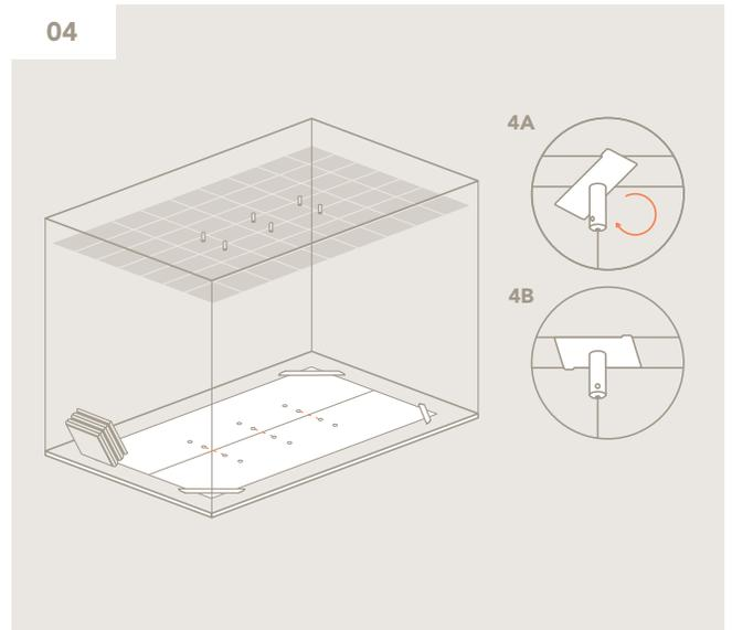
Once both points have been marked, use measurement (D) to ensure the accuracy of spacing between anchor points. Attach all the T-Bar clips to the anchor point on the grid by pressing upward and twisting (4A, 4B). Ensure the T-Bar clip is locked in place.
